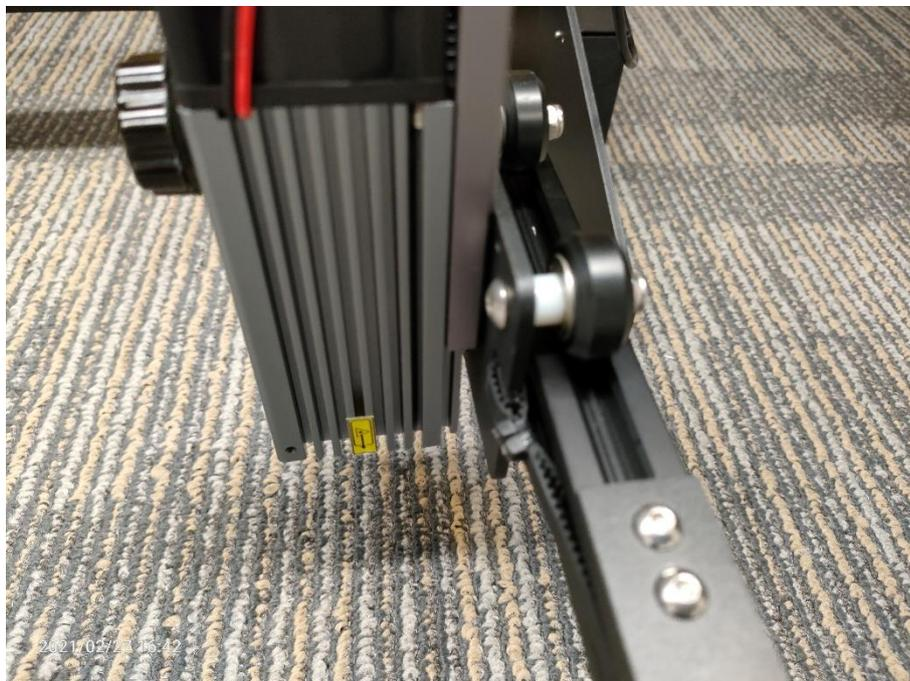
Figure 8. Laser aperture marking of model A7 30W
