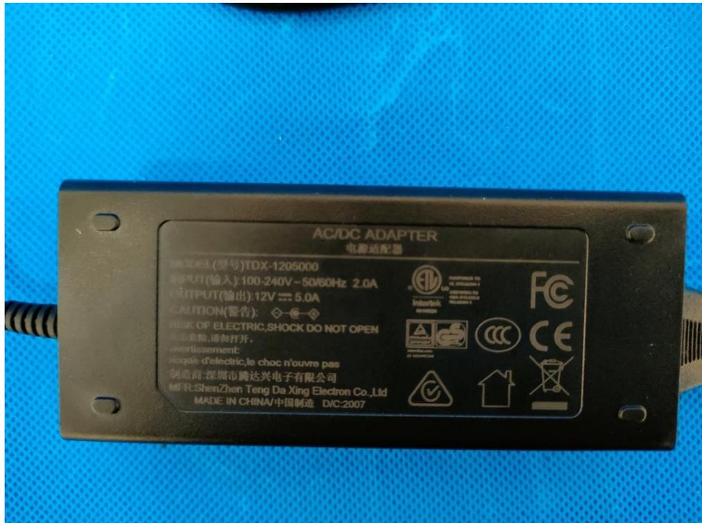
Figure 53. Rating label of AC adapter
