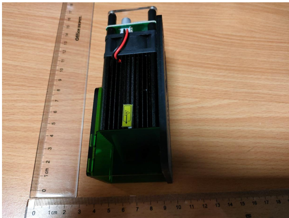
Figure 32. Laser aperture of model L40 with green plastic cover
